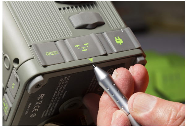
TRIUMPH-LS shown above and its slant height measurement point (SHMP). A similar mark is also on the opposite side of the TRIUMPH-LS.
