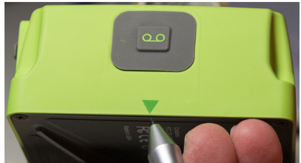
TRIUMPH-2 shown above and its slant height measurement point (SHMP).
